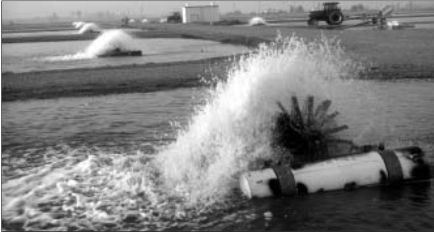
Figure 6. A series of electric paddlewheel aerators in operation.
